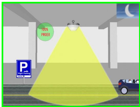
Mode 3: Full brightness continues for a set period after presence is sensed.
