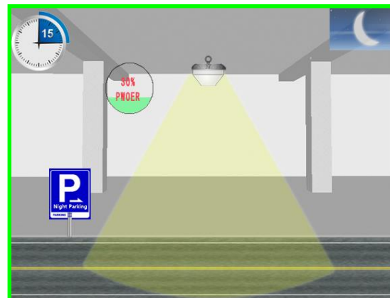
Mode 4: After a predetermined period people of time since presence is not sensed brightness returns to 30%.
